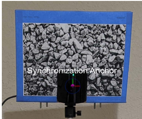
Figure 1: Vuforia image target mounted on top of Vive-Pro Base Station 2.0, synchronization anchor position adjusted down from the center of the image target to the base station center.
