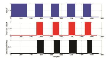
**Fig. 9.** Target indicators and resulting vector calculated by the system (example). On the top shows the original target vector. In the middle shows the improved target vector after trimming the first target and on the bottom shows the resulting vector from our approach.
